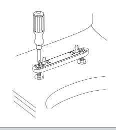
Push seat downward to Hingebase Board Assembly.
