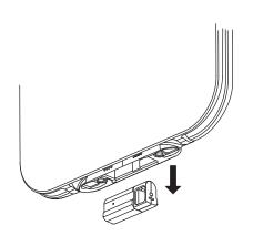
Remove film from Scent Pack install Scent Pack and 2 AAA Battery into Night Light & Scent Function Module back to seat, push seat downward to Hingebase Board Assembly.
